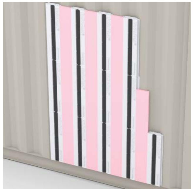
Use approximately 5" wide sheet foam when installed in every corrugation.
