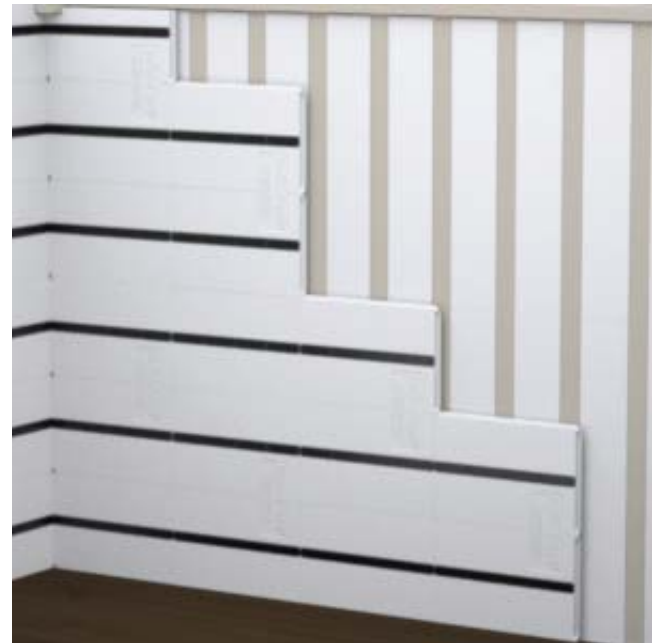
Vertical running bond pattern.
