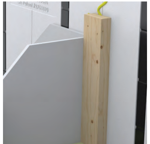
Interior wall glued to panels.
