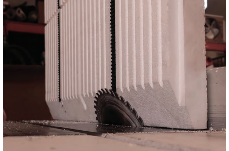
Don't cut the angle all the way through. Keep a flat area on the bottom.
