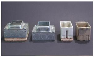
9. Install a 2-1/2" deep box, a 1 ½" deep box with a 1" mud ring or a 2" deep box with a 1/2" mud ring. Secure plastic, metal, or fiberglass electrical boxes directly to the concrete wall with adhesive or a mechanical fastener.
