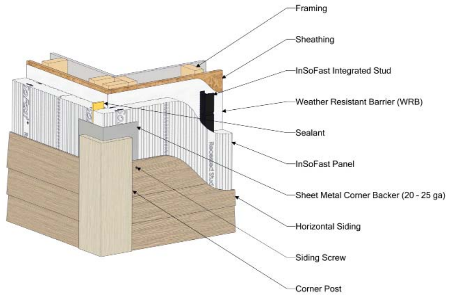
Outside Corner with Sheet Metal Backer
