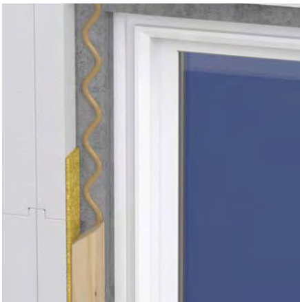
Seal between the panels and furring.
