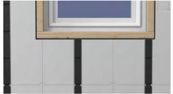
Install wood furring around openings.
