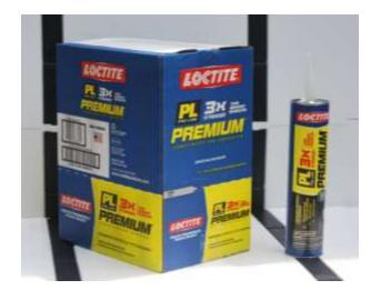
Don't be alarmed if it feels a little spongy at first. PL Premium takes about 20 minutes to set and 24 hours to cure. It can form a "liquid shim" spanning gaps of up to  $3/_8$ -in and effectively tighten up small irregularities in a wall's surface.
