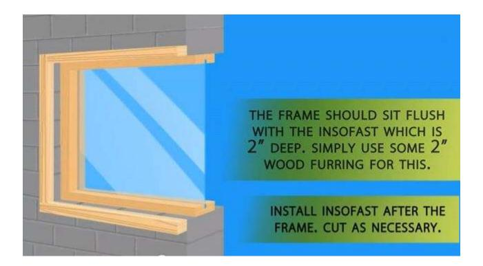
You can use pressure treated lumber, western cedar or a cellular PVC. You want to make sure that you limit the exposure of the natural wood framing coming into contact with the concrete and moisture.
